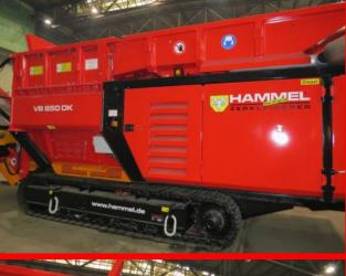
10 / 2013 construction year: operation hours: approx. 700 h drive: diesel CAT C13 approx. 475 PS power:
